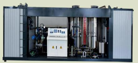
Compressed air drives fluid flow which is governed by pneumatic valve. This design saves human labor and reduces labor intensity.
