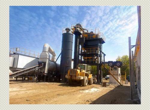
YLB Mobile Asphalt Mixing Plant
