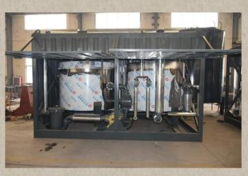
The equipment can stir the matrix asphalt, rubber powder, SBS particles, additives and the like through high-speed shearing and grinding of the shear mill, so that the modifier is fully dispersed into the matrix asphalt by chemical and physical action, and the matrix is completed. Modification of asphalt.
