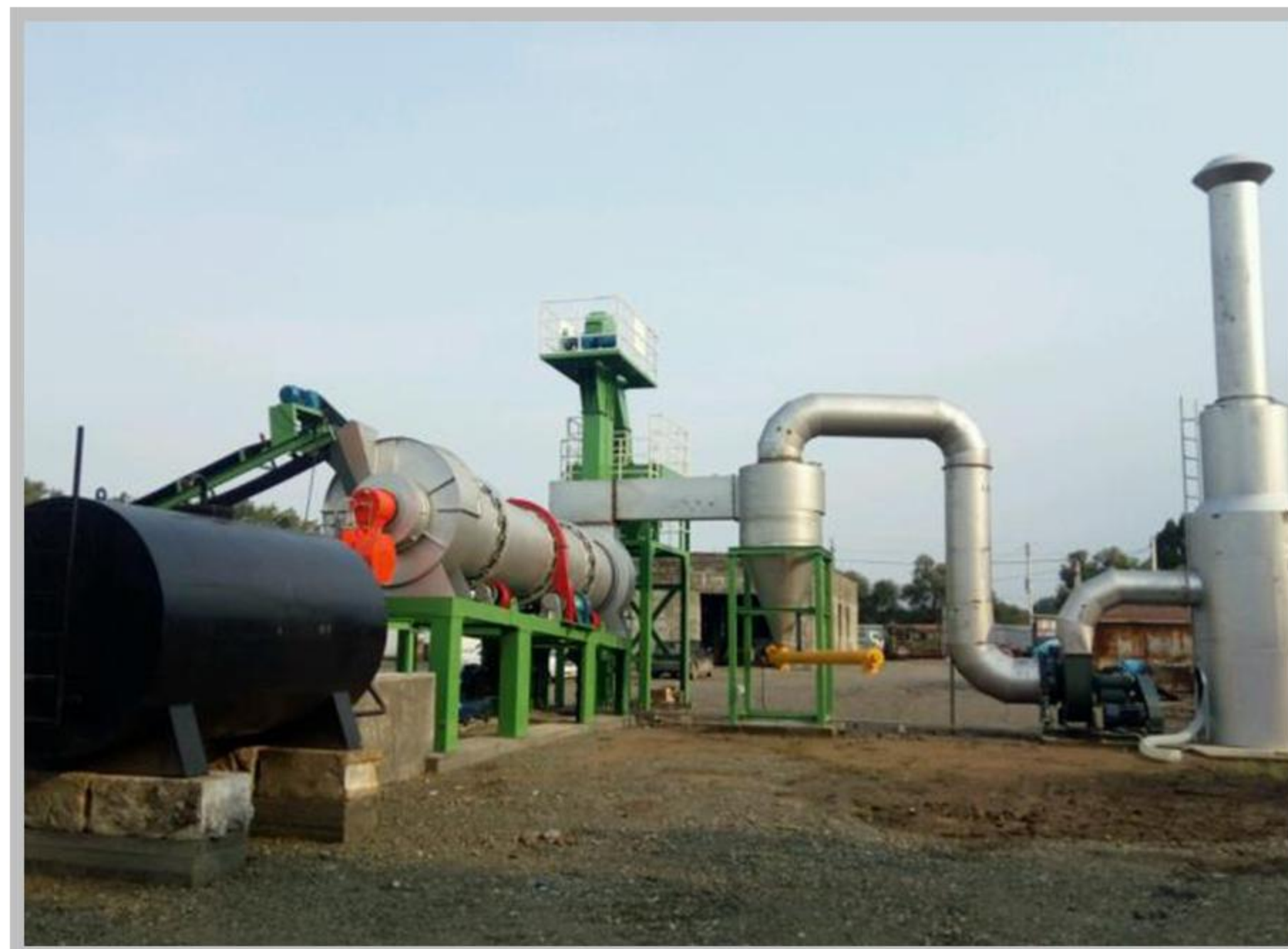
60tph continuous mixing asphalt plant in Ukraine
